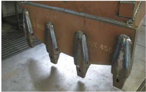
Weld with small multiple runs following the weld groove in the adapter. Place the root beam at the bottom of the groove and continue welding as shown in sequences filling up to the groove in Figure 8 by alternating between bottom and top leg at the adapter. Clean each beam before applying next pass of weld; use a hammer for slag removal and a steel brush. Welding defect such as cracks, slag inclusions, porosities, overlaps and undercuts shall be removed by grinding.
