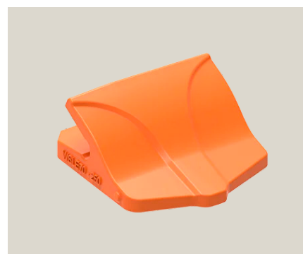
Weld-on shroud WSLE70, left Fits 60-70 mm cutting edges with 15° angle from excavating direction.
