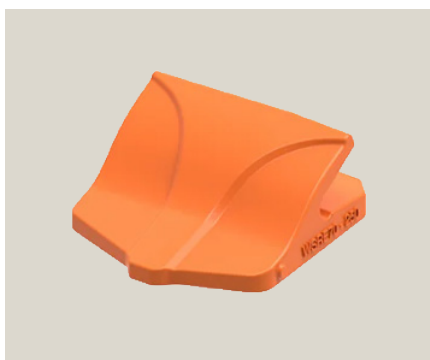
Weld-on shroud WSRE70, right Fits 60-70 mm cutting edges with 15° angle from excavating direction.
