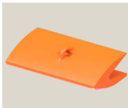
Welded shroud 16204 This shroud can be cut to length and mounted between the adapters on cutting edges between 75-90 mm thickness.
